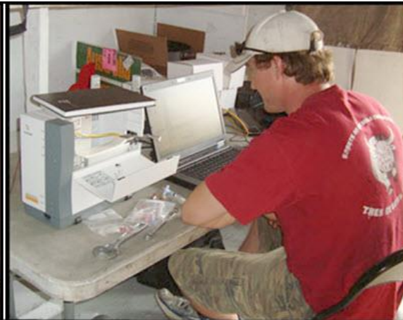
Micro-GC for Helium/Hydrogen Analysis
